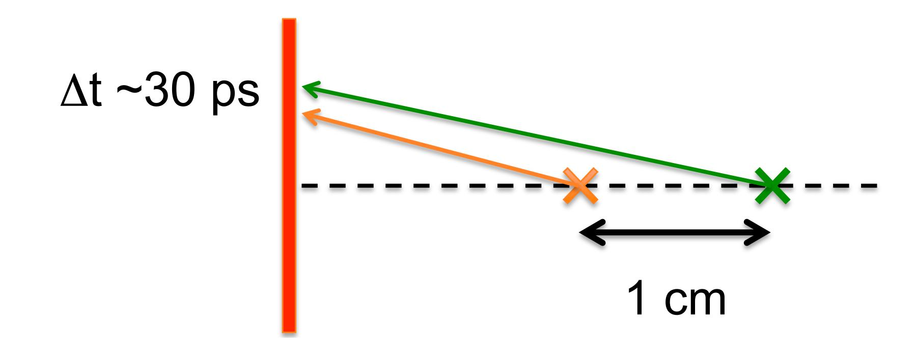
Time of flight can be used to disentangle the origin of particles as well — particularly useful for neutral particles
