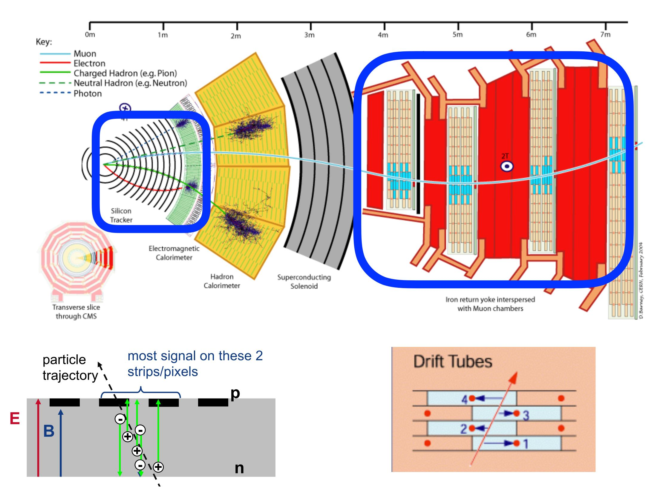
Precise, high-granularity silicon pixel and strip detectors are the workhorse
