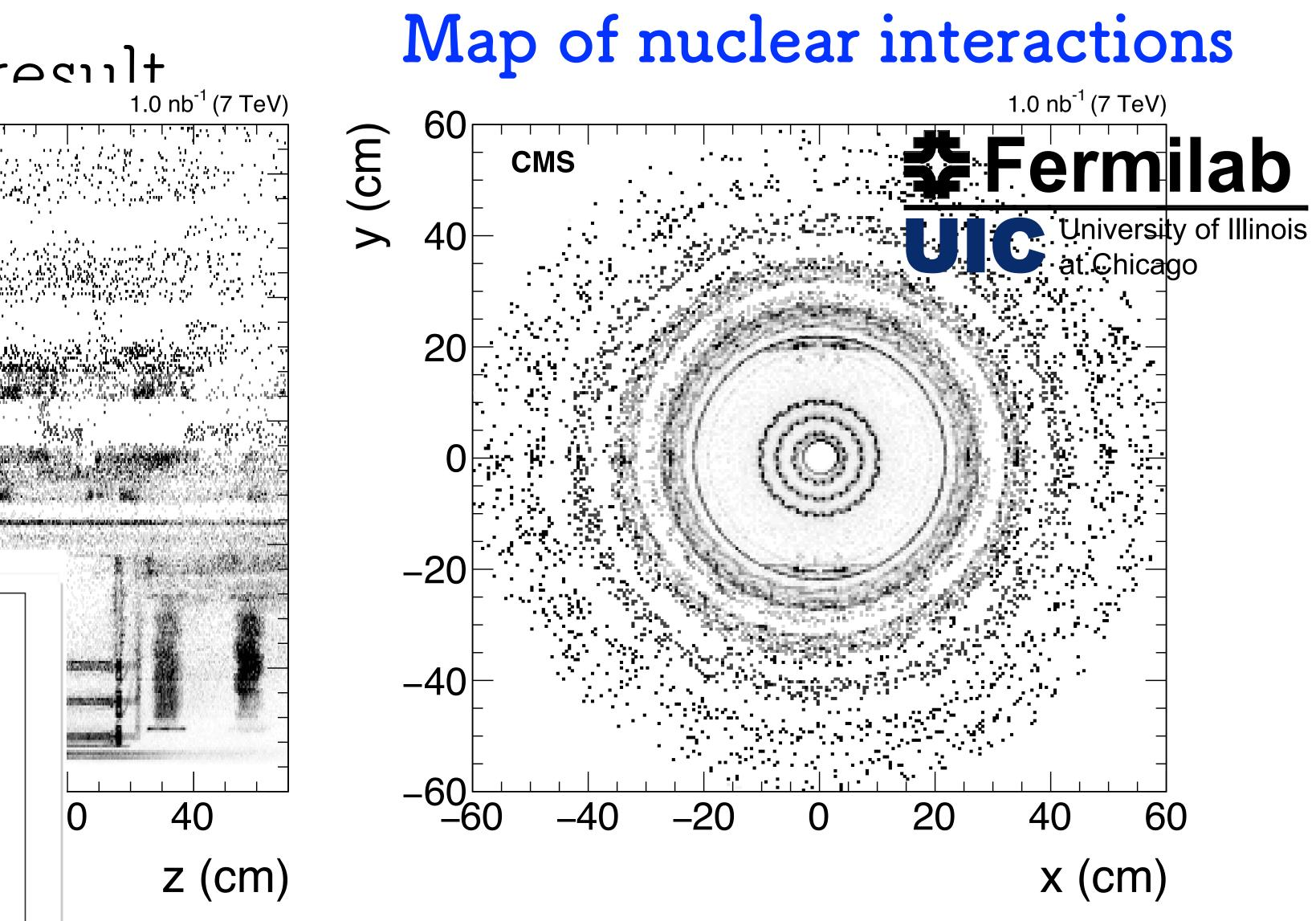
To avoid double counting, nuclear interactions need to be identified and combined into primary particles (part of particle flow, see later)
