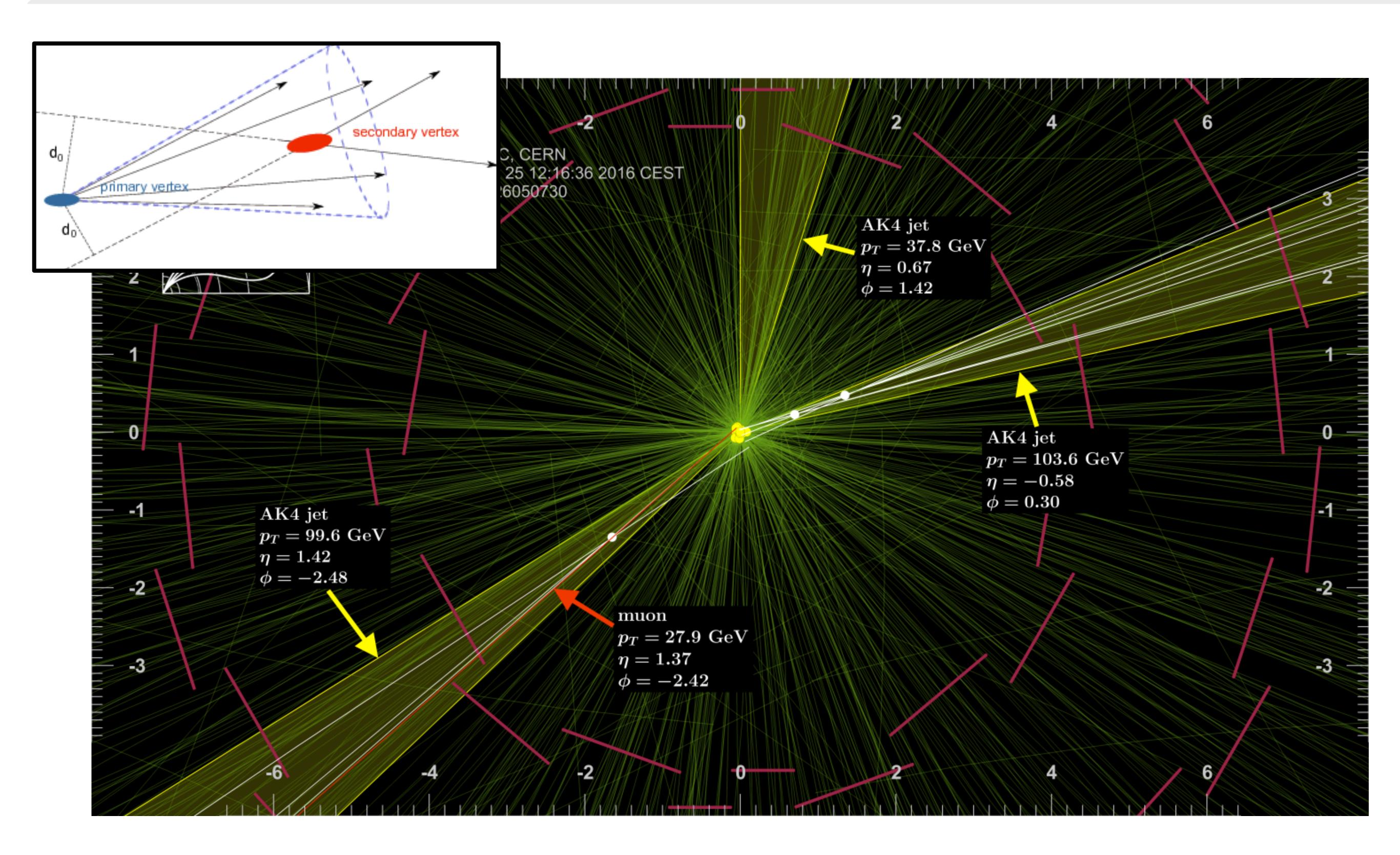
Use impact parameter of the secondary vertex to identify displaced vertices
