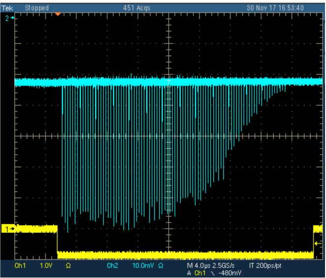
At high repetition rates, gain of MCP-PMT sags due to charge accumulation
