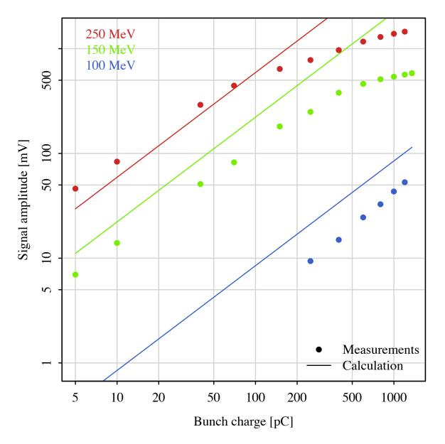
Measured signal is ~ 2 times smaller than expected at lower energies; larger at 250 MeV
