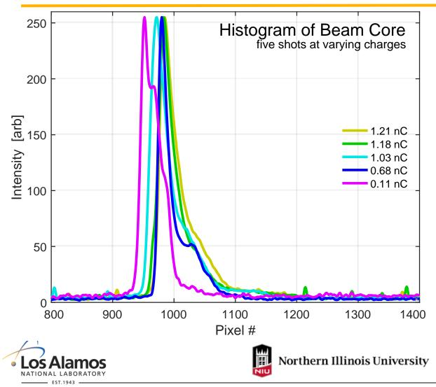
As the bunch charge varies, the beam energy fluctuated, but is not a significant problem.
