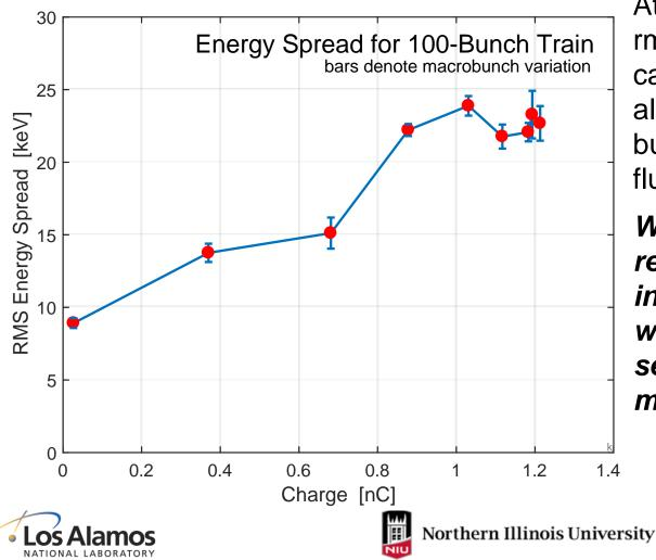
At each bunch charge, the rms energy spread was calculated. An error bar is also included to show the bunch-to-bunch fluctuations.
