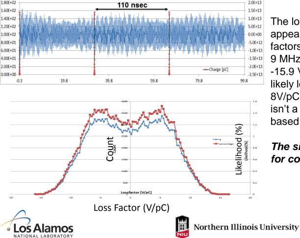
The longitudinal wake has a stochastic appearance (top). Binning of the lossfactors over a distance of 5 bunches at 9 MHz rep rate (bottom), max/min are -15.9 V/pC to +16.5 V/pC. The most likely loss-factors are in the range of -8V/pC to +8V/pC. Not clear why this isn't a normal distribution; we still based analysis on RMS approximation
