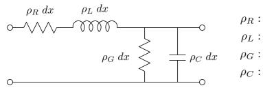
resistance/length inductance/length conductance/length capacitance/length
