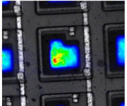
Photons are emitted during breakdown
