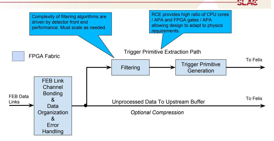
Baseline data flow in RCE doesn't touch the PS; data is received and sent out through the fabric using the high-speed IO links
