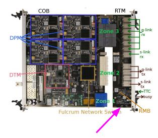
Broadcom MicroPOD transmitter/receiver supports 10.3125 Gbps per lane: http://www.fit-foxconn.com/Images/Products/Spec/AFBR-77D1SZ\_20160510175052121.pdf Experience with high density fiber optic RTMs
