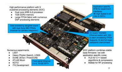
Trigger Primitive Generation: ATCA-based RCE cluster (i.e. FPGA farm)
