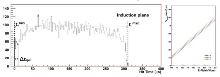
Average drift velocity using through-going muons known to better than 2%.
