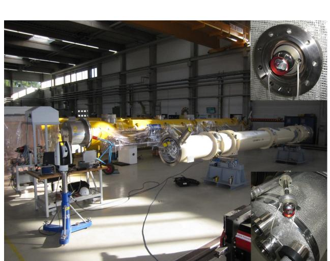
Transfer measurement of one dipole with a Leica AT960
