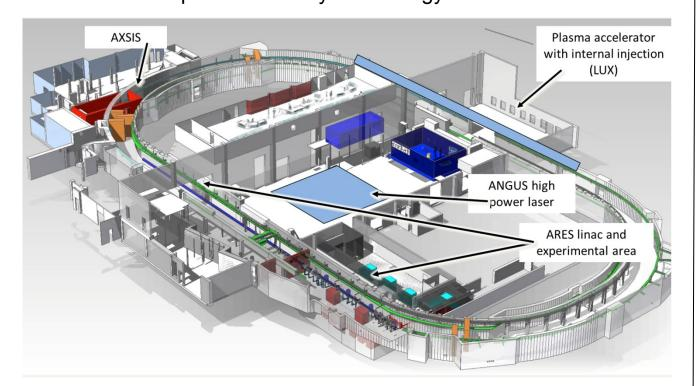
Short Innovative Bunches and Accelerators at DESY (SINBAD) is located in the building of the old DORIS ring (1974 – 2012) and contain different new types of accelerators like ARES and LUX.
