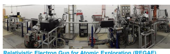
Relativistic Electron Gun for Atomic Exploration (REGAE) is a small 10 meter long electron acccelerator which works like a transmission electron microscope to directly observe the most venerable concepts in chemistry and biology.
