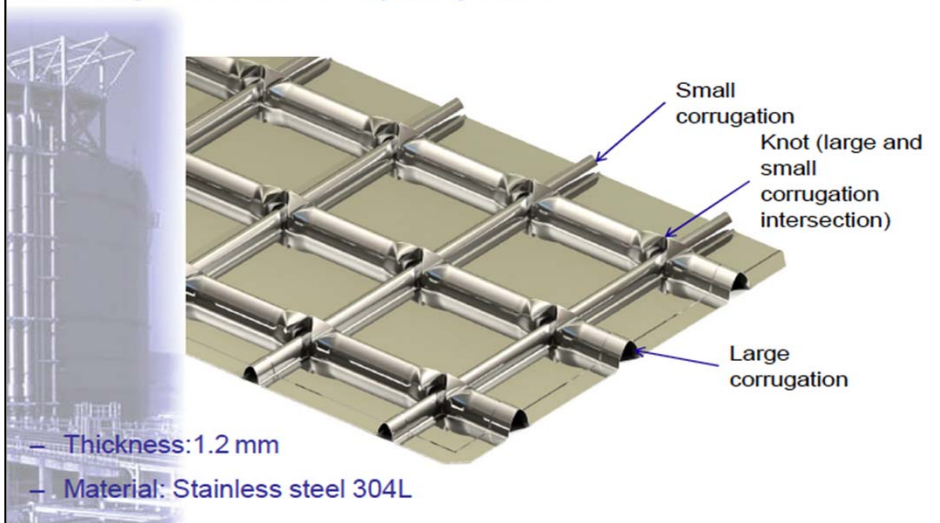
The corrugated stainless steel primary barrier:
