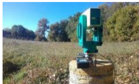
Figure 5. Mekometer ME5000 stationed on a pillar of the Long Distance Control Baseline
