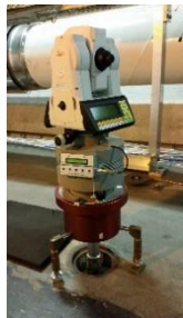
Figure 3. Gyromat 2000 stationed on a underground network reference point in the LHC tunnel
