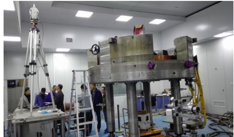
Alignment of cyclotron magnetic field measurement
