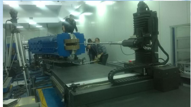
Dipole Hall probe mapping positioning
