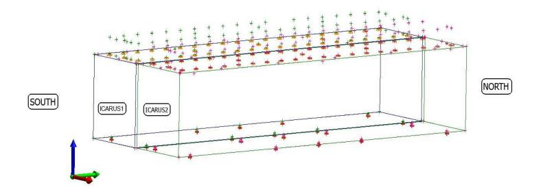
Pre-Installed Locations of ICARUS1 and ICARUS2 Detectors inside the Warm Vessel were determined by transforming the measured detectors in the parking lots into the Cold Feet centers measured inside the Warm Vessel, in the SBN-FD Building Coordinate System
