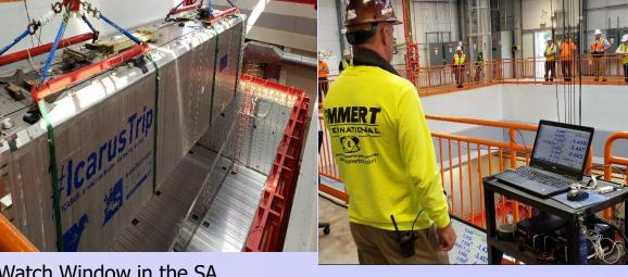
Watch Window in the SA software was used to display the measured coordinates in real time as the detector was being
