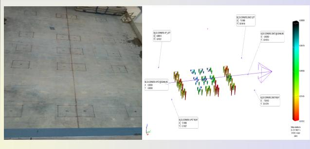
Flatness of all 20 Warm Vessel Pads measured and centered on the beam line
