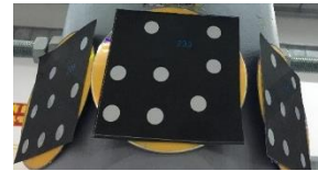
Figure 7: 3D coded target
