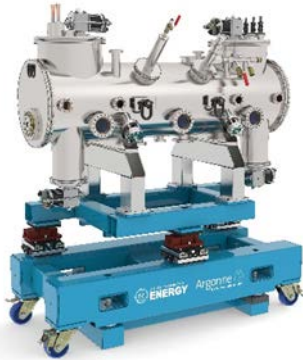
Figure 10: Photo-realistic rendering of the Helical Superconducting Undulator (HSCU) cryostat vessel
