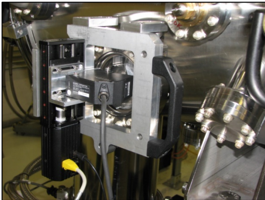
Figure 6: Photograph of the Cryoscanner instrument coupled to a cryostat vessel
