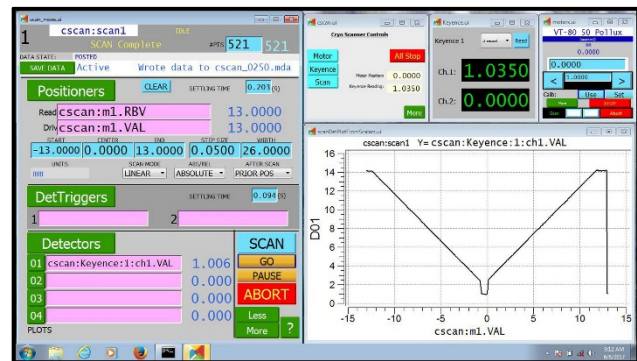
Figure 8: Screen capture of the EPICS control and data acquisition interface, including a 2-D real-time plot of a vee-block target profile
