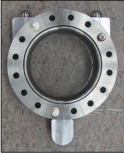
Figure 5: Vacuum flange with kinematic element modifications and viewports attached
