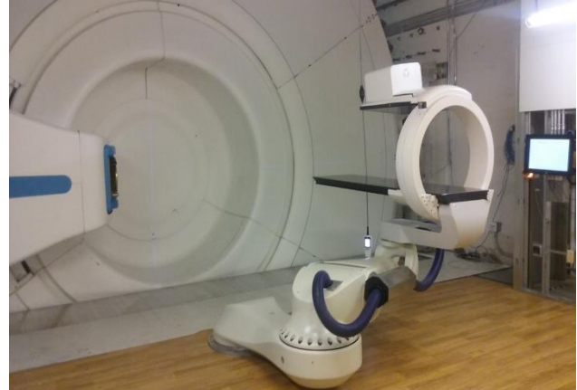
Figure 15: Leoni robot and Med Photon imaging system.
