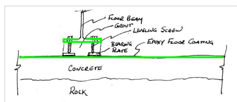
Application of Epoxy Coating to both Concrete and Steel (Belts and Suspenders) to Isolate Detector Steel and Grout from Underlying Concrete and Rock T. HAMEENIK.
