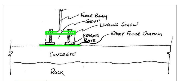
Application of Epoxy Coating to both
