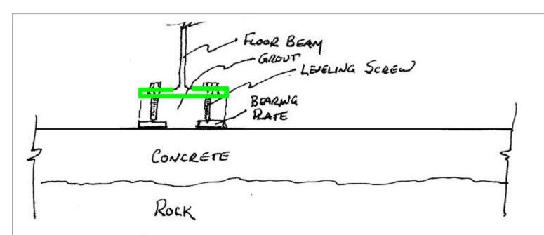
Application of Epoxy Coating to Steel Isolate Detector Steel from Underlying Concrete and Rock - Need to Address Conductive Path Through Leveling Screws/Plates (Perhaps Remove Screws after Grouting)
