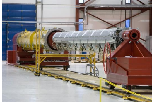
Cryomodule assembly floor of ICB Coldmass insertion to a vacuum vessel in ICB
