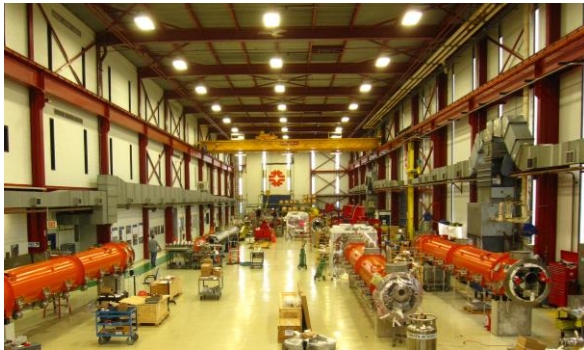
Cryomodule assembly floor of ICB Coldmass insertion to a vacuum vessel in ICB
