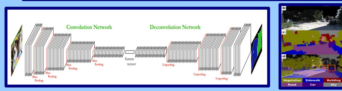
A semantic segmentation network (SSNet) associates each pixel with a particular label. i.e. a labeling network tells you the score for "dog" in this image. An SSNet will label which pixels it thinks are dogs
