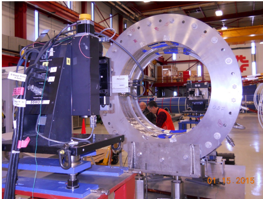
Alignment support locating the vibrating wire position of the TS prototype
