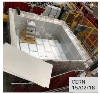
Electrical and mechanical tests of each final CRP in nominal thermodynamic conditions:
