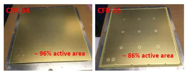
Tests performed at Saclay: CFR35 offers a safe design with an improved stability and reaches the required HV up to 3.5 kV
