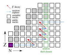
• How far can the *r* process proceed? Number of free neutrons that seed nuclei can capture (neutron-to-seed ratio).
