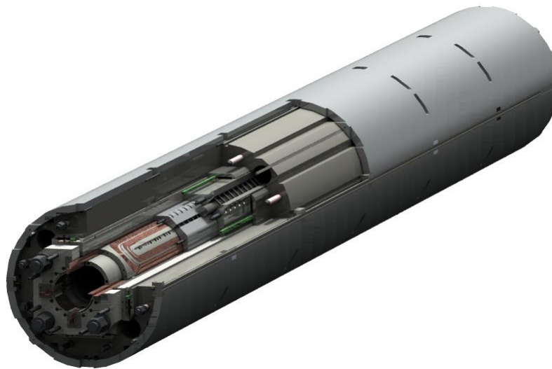
Figure 4: MQXFA 3-D conceptual cutaway view
