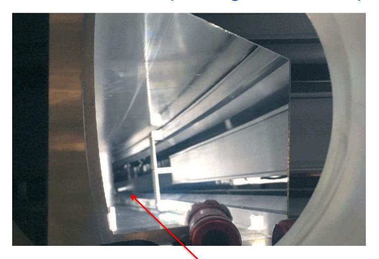
Broken horizontal ceramic standoff on Q1S inner
