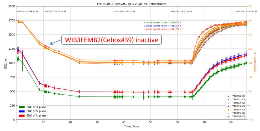
Uniform gain (77e<sup>-</sup>/bin) is applied for calculating noise of all channels
