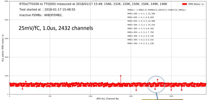
Found 2 abnormal V wires where a wire was cut (low noise) and soldered to its neighbor (high noise) All electronics channels (aside from 1 FEMB) functioned well after warmup: open channels remain
