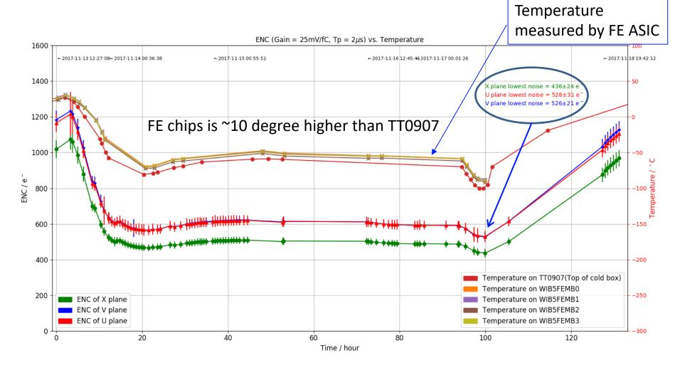
Note: Uniform gain (80 e-/bin) is applied for calculating noise of all channels
