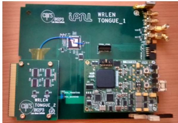
Figure 1.13: Picture of the WR slave node card (WR-MCH) present in each uTCA crate for time synchronization. The WR-LEN mezzanine card is visible in the bottom right corner
