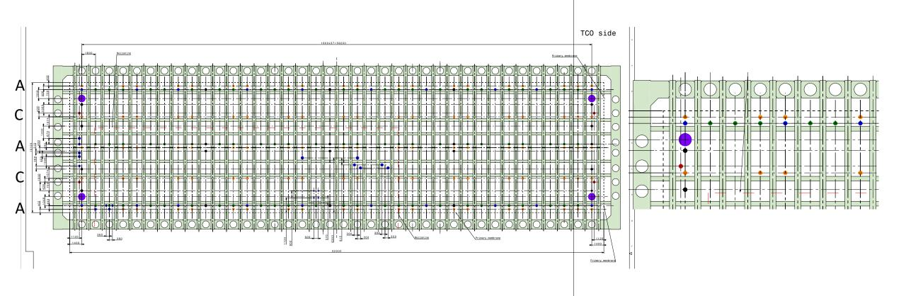
Green = TPC & PD cables; Orange = Detector Support System; Blue = Cryo
