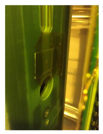
➤ Epoxied small 0.5 cm thick G10 pieced above screw heads on the side of the frame. The heads were supposed to remain inside of the frame, but some of them sticks out, potentially risking to make electrical contact with the neighbor APA (3 mm gap between APAs). This fix the problem
