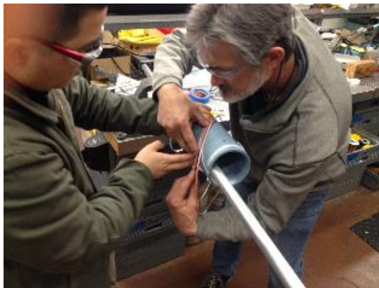
Hugh Higley (left) and Andy Lin (right) winding a 40-turn mockup coil
