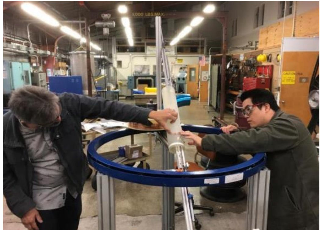
Hugh Higley (left) and Andy Lin (right) winding a 40-turn mockup coil
