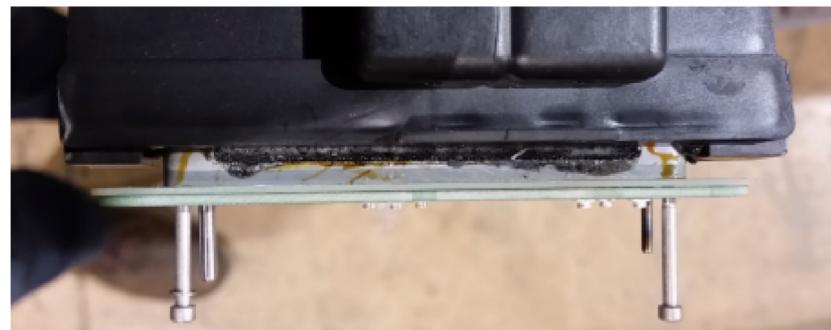
Prototype SiPM board attached to module snout.
