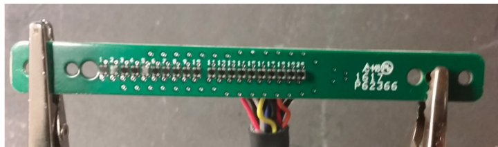
Prototype SiPM boards fabricated at CSU.
