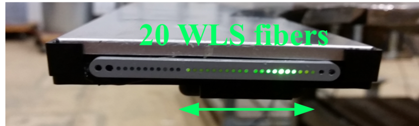
MINOS module snout with 20 fiber ends (same on the other end).
