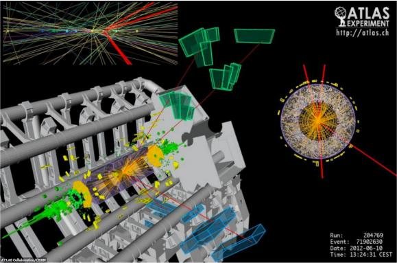
A four-muon candidate event in the ATLAS detector at the Large Hadron Collider. The muon/anti-muon tracks are highlighted in red, as the long-lived muons travel farther than any other unstable particle.
