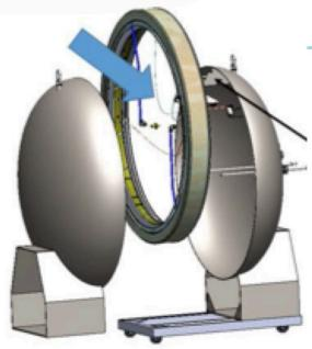
From last week: GA cryostat for testing the model coil. The coil will be mounted horizontally in the cryostat and cooled to liquid nitrogen temperatures to test for mechanical stresses. The coil will then be shipped to Fermilab for destructive test to look for voids in the VPI and stress fractures from the cold test.
