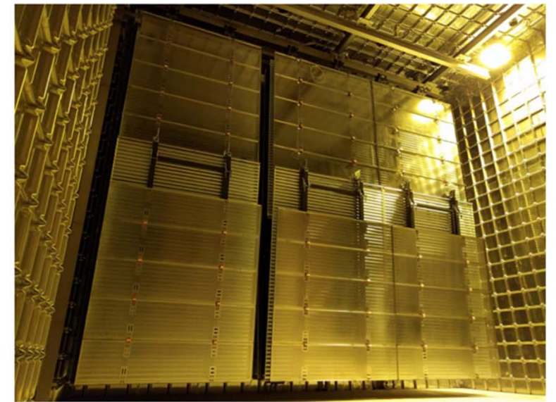
Above: APA1-3; below: CPAs & top/bottom field cages
