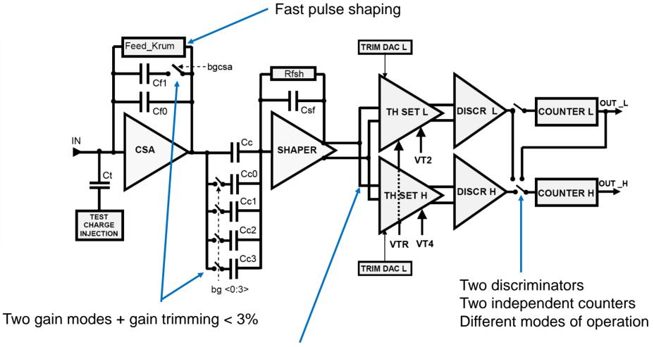
Precise offset trimming < 10 el. rms
