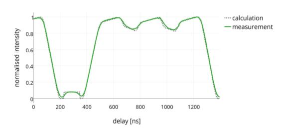
**Figure 5**. The hybrid filling mode of SOLEIL storage ring measured with the UFXC32k detector (green line) and calculated from the actual machine current values per packet (grey-dashed line). The measured scan was obtained by illuminating the detector with Ge fluorescence radiation ( $K_{\alpha} = 9.9 \text{ keV}$ ), and registering a large number of frames of 120 ns with precisely controlled delay with respect to the storage ring clock.
