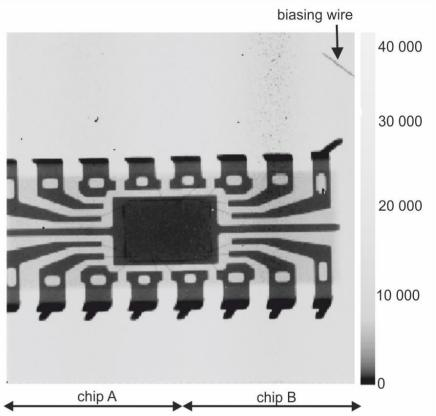
An example of DIL radiogram acquired with the fully assembled 2-chip module.
