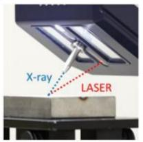
Arrangement of head unit and sample
