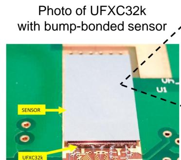
32768 pixels (75x75  $\mu$ m<sup>2</sup>) CMOS 130 nm (~50M transistors) chip size 9.63  $\times$  20.15 mm<sup>2</sup>
