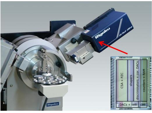
Replacing a conventional scintillation counter with D/teX Ultra on an in-house X-ray diffraction (XRD) system, one can reduce the data acquisition time by 1/100, or improve the sensitivity 100 times when the same data acquisition time is applied.
