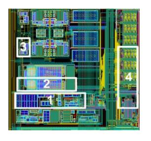
Layout of a pixel – **pitch 100 um:** 1 – CSA, 2 – Threshold setting block, 3 - Discriminator, 4 – Counter and logic
