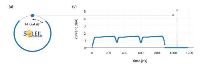
**Figure 3**. The hybrid filling mode at SOLEIL: (a) schematic view and (b) time-distribution of current per packet.
