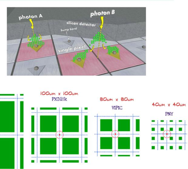
The first solution of this problem was proposed by CERN and consequently it was implemented in the Medipix III chip. However, due to pixel-to-pixel threshold dispersions and some imperfections of the simplified algorithm, the hit allocation was not functioning properly.
