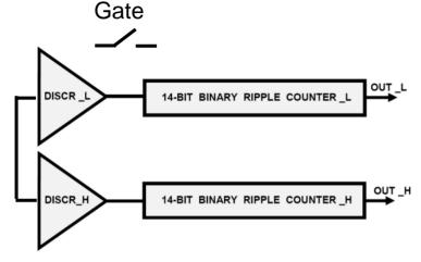
Standard Mode (Energy Window): DISCR\_L ⇒ COUNTER\_L (N bits) DISCR H ⇒ COUNTER H (N bits)
