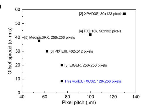
Offsets spread in large area integrated circuits working in the single photon counting mode vs. pixel pitch – reference and pixel matrix size is speficied for each solution.
