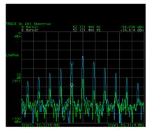
Figure 5: Frequency spectrums of gap voltage monitor on one of the eighteen cavities. Blue and green traces show signals without and with feedforward beam loading compensation. The vertical scale is 10dB/div.
