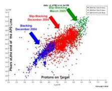
Figure 9: Number of pbars in an ion chamber after the target as a function of the number of protons on target. Blue points are with non slip stacking in December 2004, red is with slip stacking in December 2004, green is with slip stacking in March 2005.
