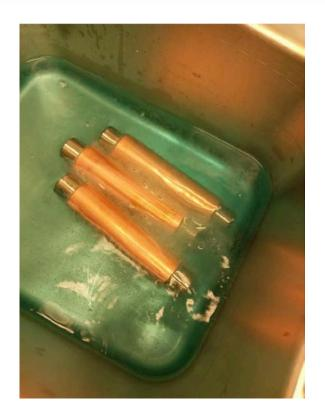
Cleaning of three other tower heat exchangers (FNAL custom) was completed at Northwestern using "piranha solution"
