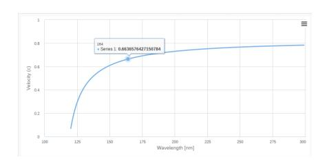
group velocity is equal to the phase velocity vp=c/n only when the refractive index is a constant
