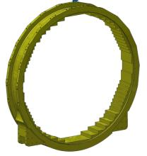
Outer monolithic C-profiled ring is machined from a block of Al 6082 to achieve maximum stiffness (max def. 4 microns).
