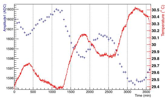
Note: Bottom plot clearly shows a negative temp coefficient
