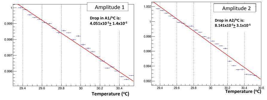
A linear fit on the temperature Vs. amplitude plots – gives the approx. gain drop / °C
