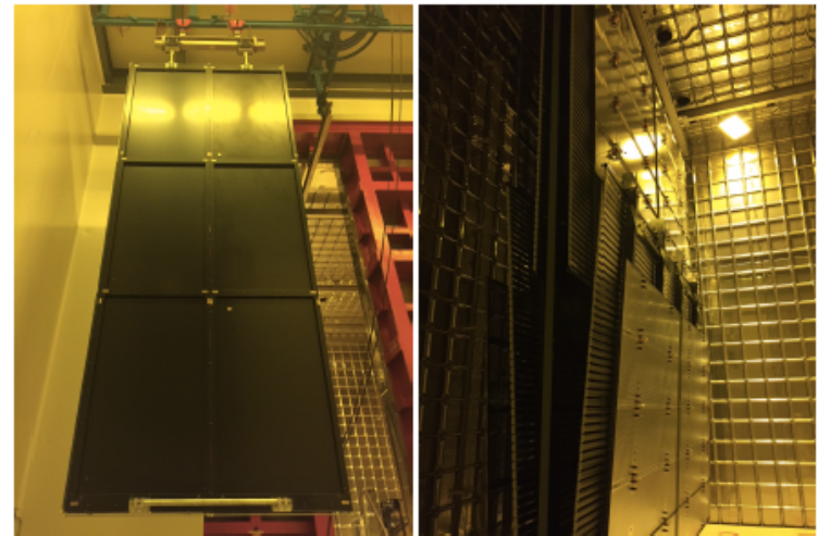
Figure 4.18: Left: Completed ProtoDUNE-SP CPA plane ready for FC attachment. Right: Two completed CPA-FC assemblies in the ProtoDUNE-SP cryostat. The top and bottom FCs with their GPs attached are visible to the right of the cathode plane in their folded-up pre-installation position.
