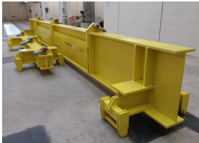
PS and DS lifting fixtures at FNAL
