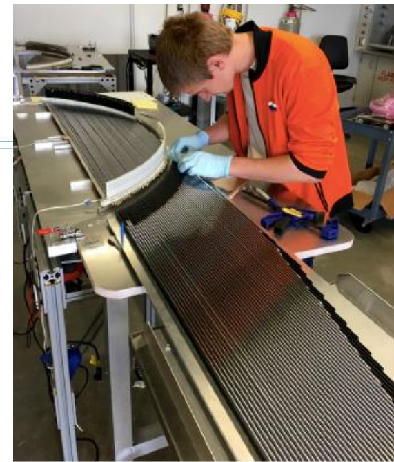
Panel: Straw Installation
