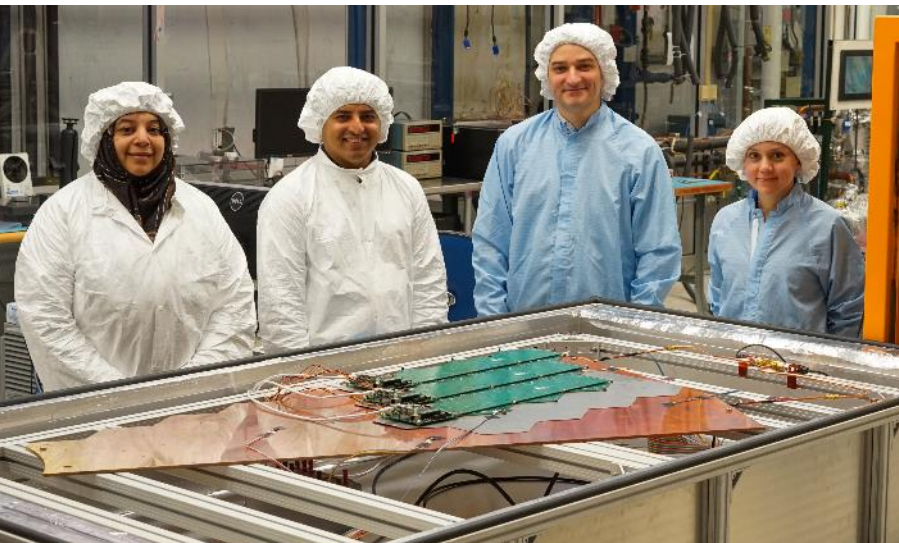
Texas Tech students Sonaina Undleeb and Kamal Lamichhane , with Zoltan Gecse and Maral Alyari testing the prototype Endcap cassette at SiDet
