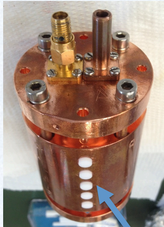
Resonant cavity with 5 GaYIG spheres inside
