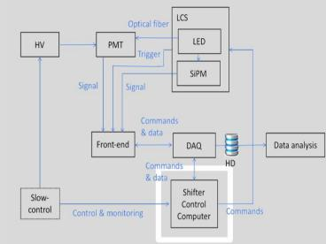
This module is in charge of coordinating all the systems involved in the LCS operation. Three different sets of commands are sent from the shifter control: to the HV (or slowcontrol), to the LCS, and to the DAQ. The format of these commands has to be the defined by the receptor subsystem.
