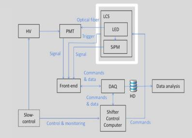
The LCS software will allow operating at different LED bias voltages and select each LED as well as the number of pulses and pulsing frequency. The software will be installed on a BeagleBone board accessed via Ethernet. the SiPM output will be connected to the light readout front-end. For each run, a text file will be generated with the internal measurement of the LED light detected by the SiPM and optionally sent to the shifter control computer.
