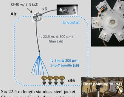
Six 22.5 m length stainless-steel jacket fibers are used inside the cryostat, each one attached to a 1 to 7-fiber bundle so one fiber is finally installed pointing at each PMT
