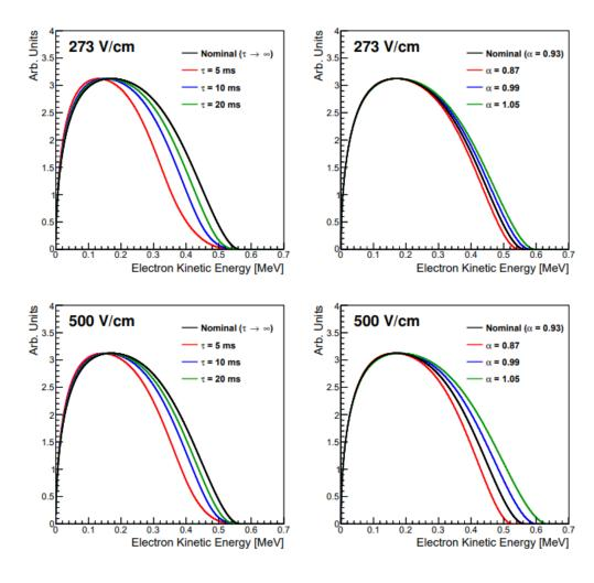
The effects of electron lifetime and electron-ion recombination are distinctly different on the <sup>39</sup>Ar Spectrum
