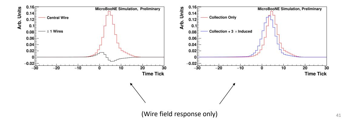
• The observed effect is explained by simulating induced charge effects (even on collection plane)
