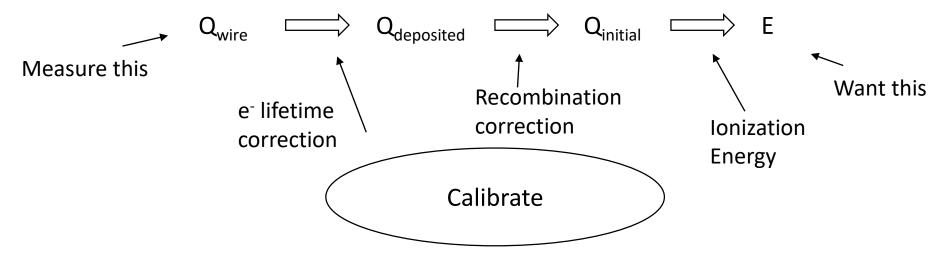
Electron lifetime correction is an important step for accurate calorimetry
