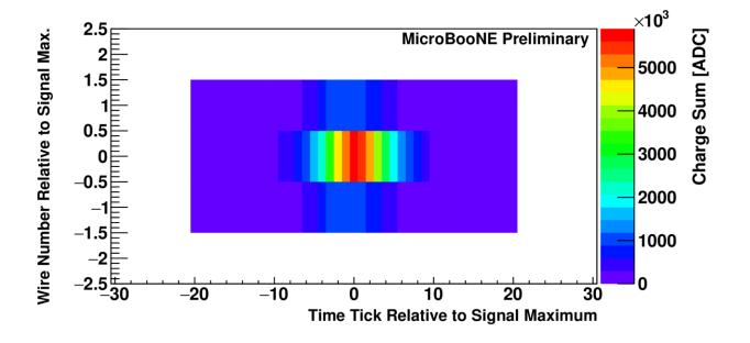
Point-like signal has applications outside of measuring electron lifetime
