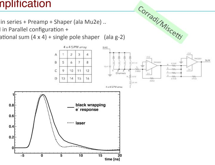
For Mu2e-II  $\rightarrow$  BaF<sub>2</sub> + SiPMs matched with the g-2-like solution is favored
