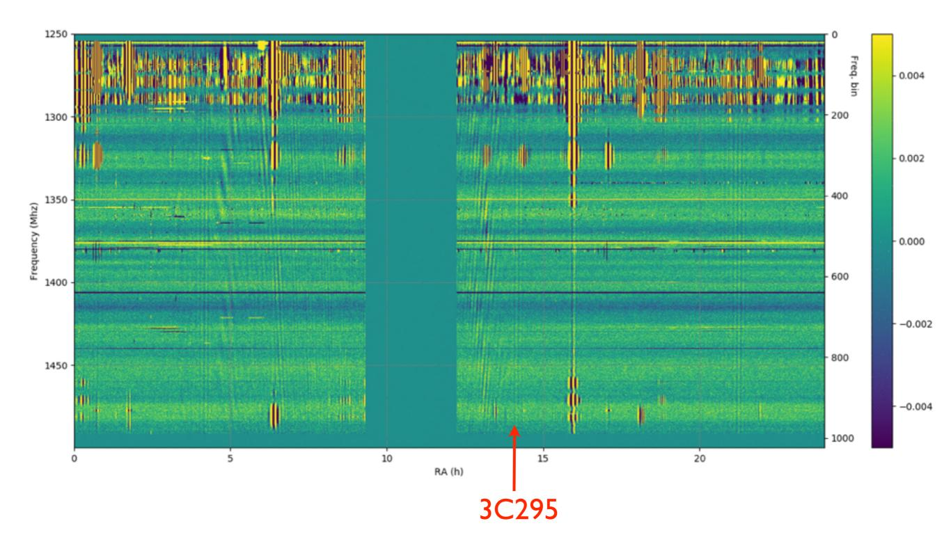
Example of time-frequency map (after gain g(v), G(t) and phase correction) - 3C295 (~ 20 Jy) is visible
