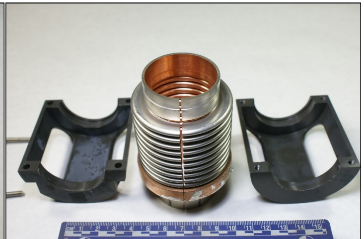
Photo 2: Bellows assembly disassembled showing the bellows with an previous EDM cut
