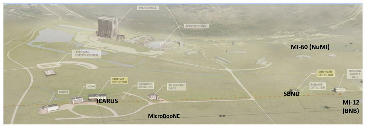
NuMI beam signals are generated at MI-60 BNB beam signals are generated at MI-12 An infrastructure of single mode fibers (SM) has ben implemented to distribute beam signals' timestamps between the various location via the WR network
