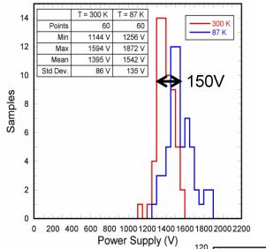
A gain variation was experienced for almost all the 60 units at 87K, with a mean reduction of ~50%. An increase of the HV supply (150V) is enough to restore the nominal value.
