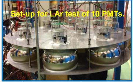
Test carried out by illumination of the PMT surface by means of a LASER diode (405 nm) and optical fibers. A standard electronic chain (PRE+AMPL+MCA) was adopted.
